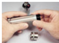
For C-cell conversion, remove the recharging module and rechargeable battery; replace with two C-cell batteries and converter.
